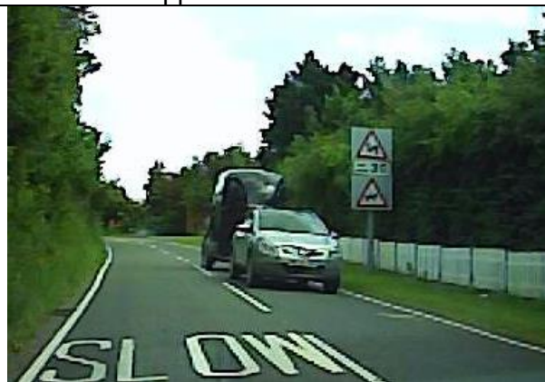
Image 6 – Larks Hill Road eastbound; bend warning sign, (with 'max speed 30mph' text) and horse warning sign on grey backing board
